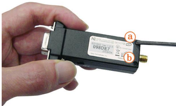
Figure 2-5 Remove ZS10 bottom cover
